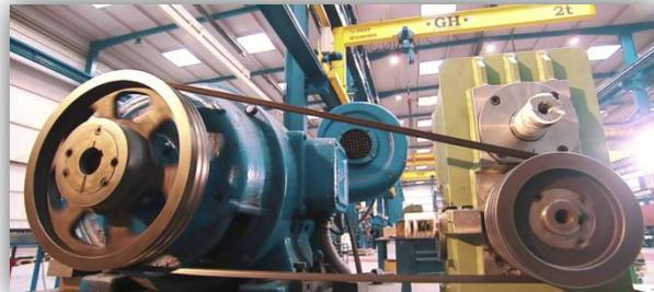
The Smart Sensor and Clutch-brake unit (left) for industrial equipment (right)
