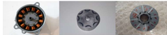
An electric motor (left) as used in millions of car's gearboxes, was chosen by the Fraunhofer team as one of their benchmark. The permanent magnets (rotor with quarter ring magnet, centre, rotor as flux collector, right) built into them contain rare earths. The Fraunhofer researchers significantly reduced the need of rare earths using a combination of different approaches.
